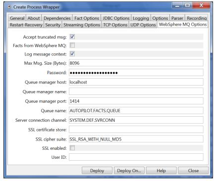
Figure 4-43. WebSphere MQ Options for JBDC Configuration
