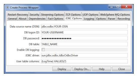
Figure 4-44. User table columns of JBDC Process Wrapper
