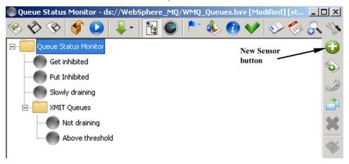
Figure 4-78. Adding New Dynamic Sensors
