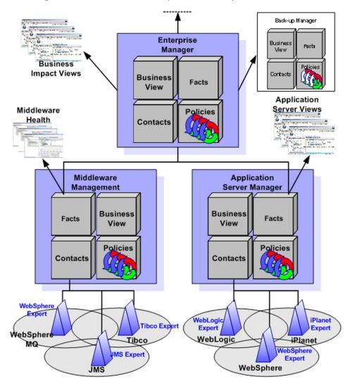
Figure 2-11. N-Tier Service Oriented Architecture
