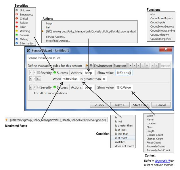
Figure 4-75. Sensor Rule Inputs
