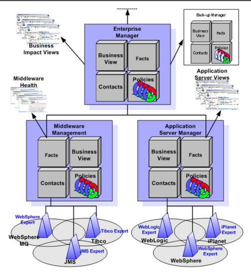
Figure 2-11. N-Tier Service Oriented Architecture
