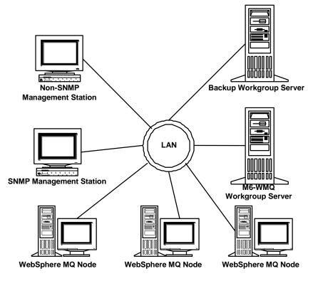
Figure 3-2. Fault-tolerant Management of WebSphere MQ
