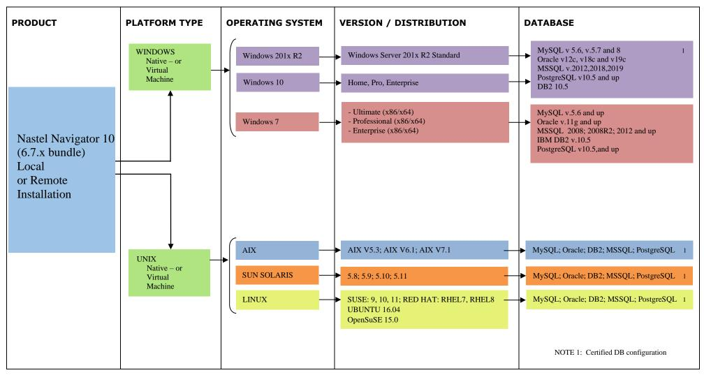
Figure 1-1. Nastel Navigator Installation Support (32-bit/64-bit)
