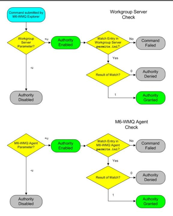
Figure 8-1. Two-level Security Checking by M6-WMQ
