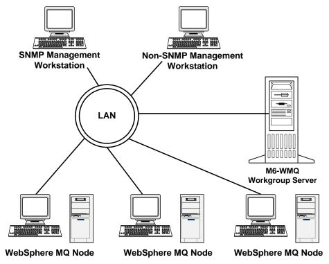
Figure 3-3. Using M6-WMQ for SNMP-based Management of WebSphere MQ
