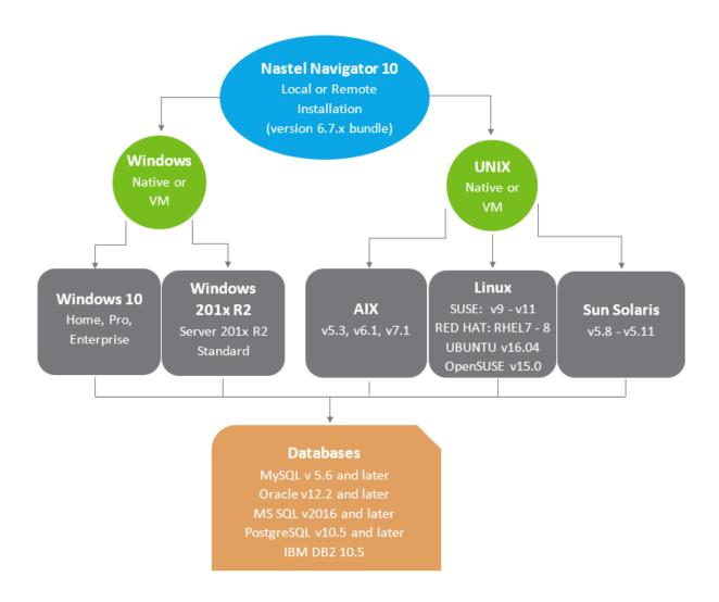
Figure 1-1. Nastel Navigator Installation Support
